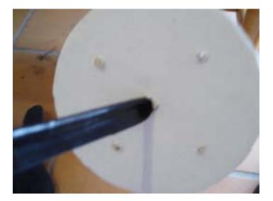
Then, gently push this disc down the mine can, so that the match goes down through the middle of the lift disc to the lift powder like this:
